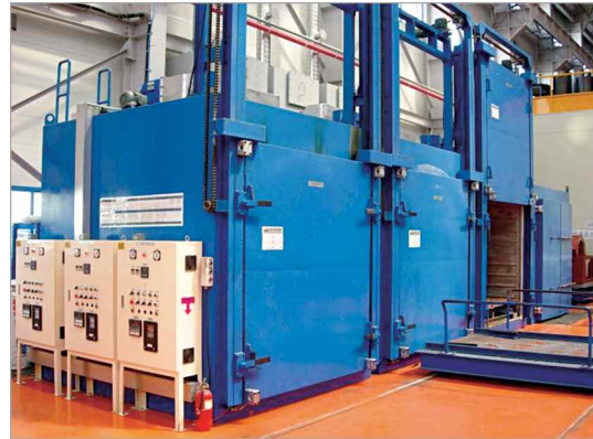
Dry Plant Electrical Heater (14 Sets)
