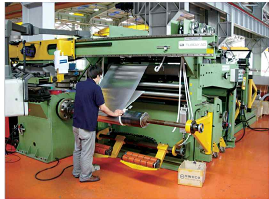
Low Voltage Winding M/C Maker : TUBOLY, H.F. STOLLBERG (3 Sets)
